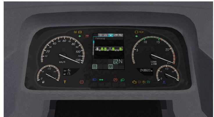
In contrast to the older monochromatic and well-arranged displays, a new small colored display was introduced. There are several check lights scattered over the panel, while some icons are also shown in the display.
