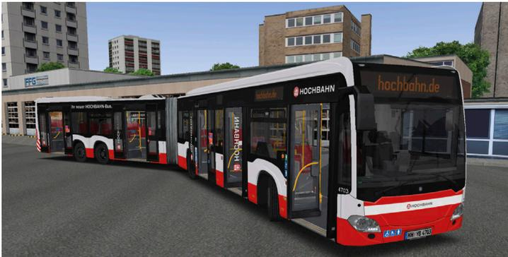
The four-axle 70-ft articulated bus has some distinctive features. The rear car is equipped with four exterior cameras on the sides and rear sides (non-functional in OMSI). The fourth axle actively supports the steering by hydraulic controls based on the front steering angle and articulation angle. Several USB charging ports have been installed in the passenger room. The front is built in the smooth uniform overland style.
