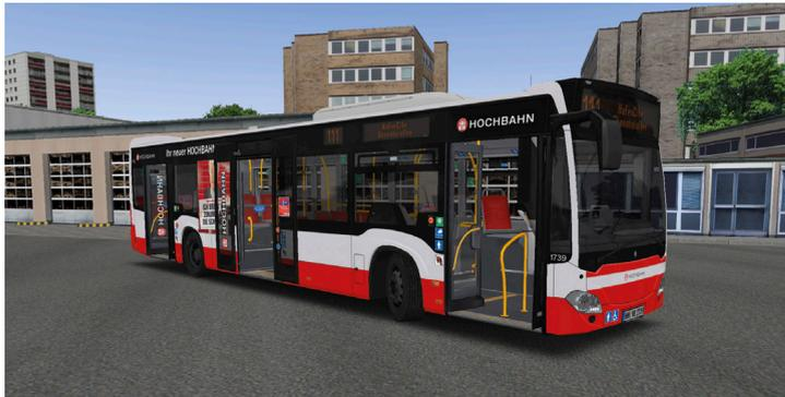
The solo bus is based on the 17 model of HOCHBAHN. Like all newer solo buses, it is fitted with three doors, with the middle one being an exterior sliding door. The transmission is a 4-speed automatic and a saloon style passenger gate is installed at the front entrance as a replacement for the older double-swing gates.
