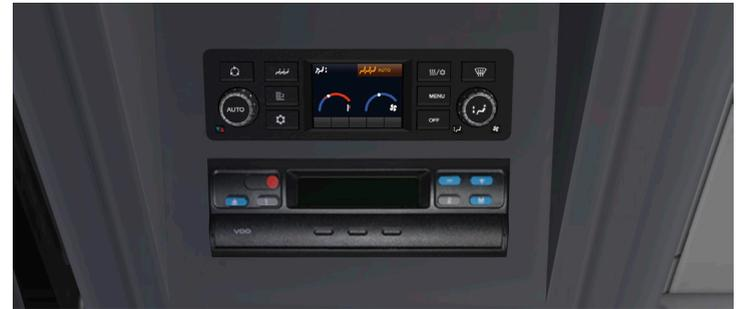
The saw tooth panels above the driver's place contain a digital trip recorder (not functional) and the A/C panel (see A/C control).
