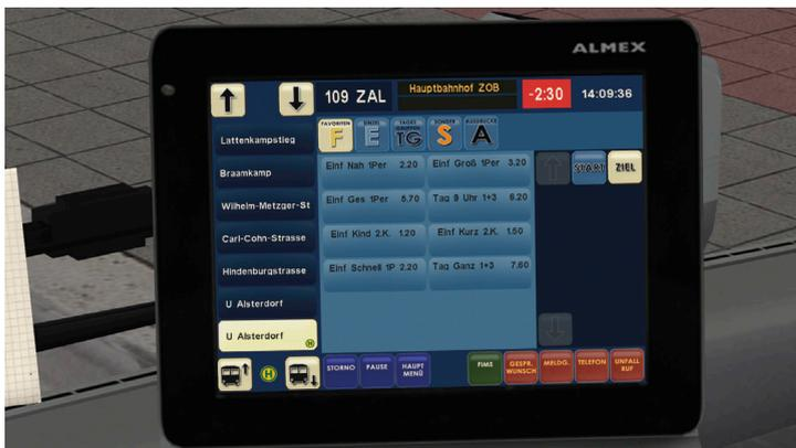
The ALMEX ticket printer ("EFAD 2") is a highly advanced touchscreen device that was developed in cooperation with HOCHBAHN. It sells tickets, controls the target display, interior stop display and plays station announcements.
