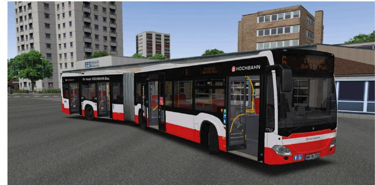
There are just 5 "model 77" articulated buses, all based in the Hamburg-Harburg depot. They are equipped with 4 doors, the second one being an exterior sliding door. It features the larger air-conditioner like the solo bus. The transmission is a 6-speed automatic.
