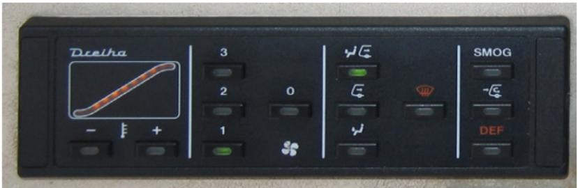
You can control blower intensity using the buttons 1 to 3; the second and third position is only available while the engine is running. You turn the blower off by pressing the 0 button. As soon as the blower is active you can set the temperature using the "-" and "+" button on the far left. Usually the front blower is using outdoor air; press "Smog" if you only want to use circulated air and press the button in the middle to use a mixture. DEF is short for "Defrost" and heats the windshield.
