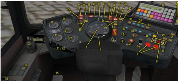
(1) Tachometer in km/h and the clock
