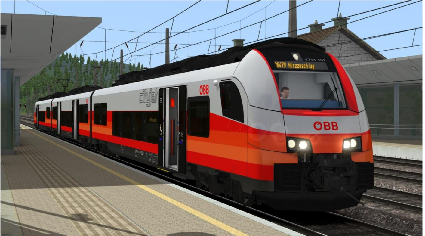
The ÖBB 4744 series (Cityjet) is an electrical multiple unit which is being produced by Siemens since December 2015.
