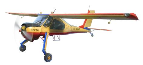
The PZL-104 Wilga was developed by the Development Design Office of the PZL factory (Poland). It was designed to be a sturdy and simple aircraft able to operate from small unpaved runways. The high wing has additional lift surfaces so it is a real STOL (Short Take-Off and Landing) aircraft that can fly at very low speeds and has very gentle stall characteristics.
