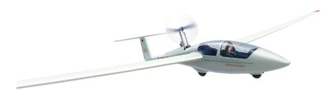
The ASK 21 Mi has a small engine delivering 41 kW. This is enough to allow the ASK21 Mi to take off eliminating the need for a tow aircraft and extending the cross-country capabilities. However, that does not mean this is a motor glider in the original sense of the word. The ASK21 Mi is classed as a 'motorized glider'. Like the ASK 21 it is a durable and robust aircraft, easy to fly and handle on the ground, you do not need any person to hold your wing.
