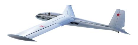
This two-seater trainer has been for many pilots the aircraft they got their first flight in. It is used all over the world with over 3000 aircraft build since 1958. Even though it is a Czech aircraft, the US Airforce (and many other Air Forces) used it for a very long time for basic flight training (under the TG-10C name). The Blaník has exception good low speed handling with effective rudders control. It is highly forgiving.
