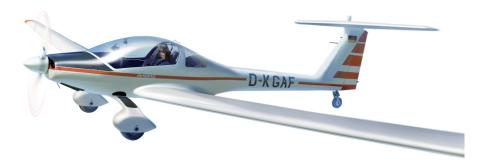
The Hoffmann H36 Dimona is not your regular small aircraft. It is in the rather exclusive class of touring motor gliders; aircraft that are a cross between motor aircraft and gliders. They got the long wings of a glider but a standard (though often rather small) aircraft engine. You can either use them as a normal aircraft or switch off the engine and glide for a while.
